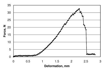
Figure 2. Example of force-deformation curve generated by materials testing unit used to determine anterior cruciate ligament stiffness and failure load.
