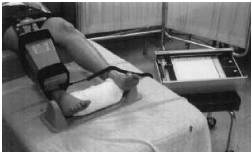
FIG. 1. KT-2000 knee arthrometer (MEDmetric, San Diego, CA) applied to subject's knee. Note the addition of a towel between the subject's feet to help maintain neutral hip and tibia rotation during testing. The compliance index used to determine ligament stiffness is drawn on the X-Y plotter at right.
